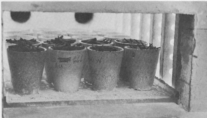
FIGURE 11. — Fireclay crucibles with contents shown in furnace, with two rows of shielding crucibles in foreground.
