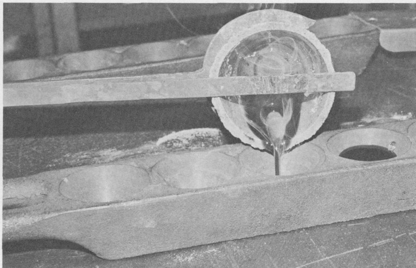
FIGURE 12. — Melt being poured into iron mold, using crucible-scorifier tongs. Note opaque glob of molten lead in crucible, which will constitute the button upon solidification.
