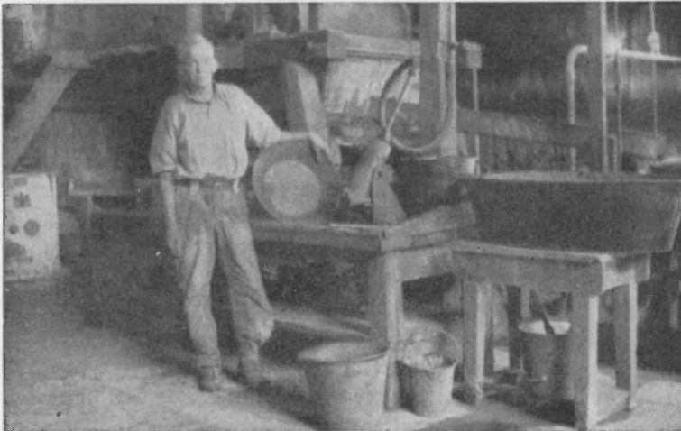
Fig. 16. Amalgamator beside his Panning Table, showing Equipment he uses for Separating Amalgam from Sand.
