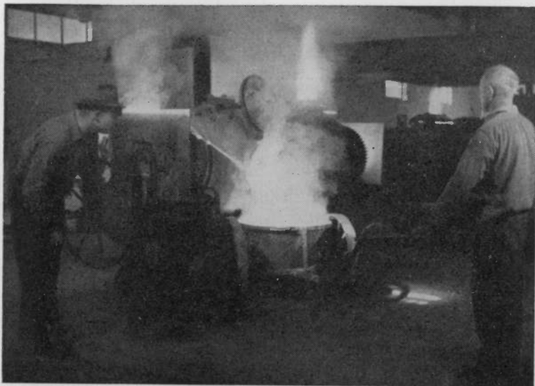
Fig. 11. Pouring Matte and Bullion from the Wabi Furnace.
