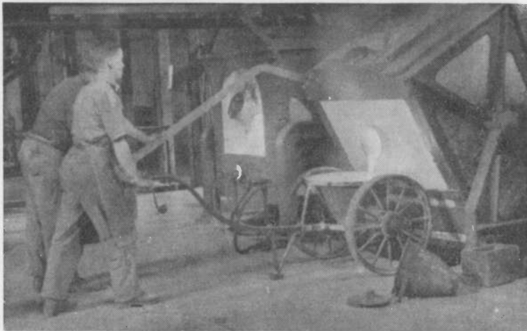
Fig. 5. Pouring a Faber du Faur Tilt Furnace. Small conical Mould shown beside the Furnace.
