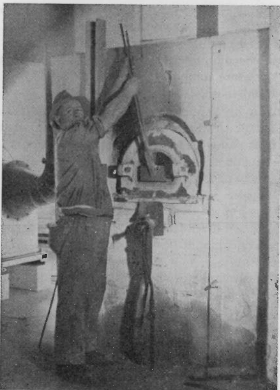
Fig. 17. Lifting Retorted Amalgam from Retort Furnace.
