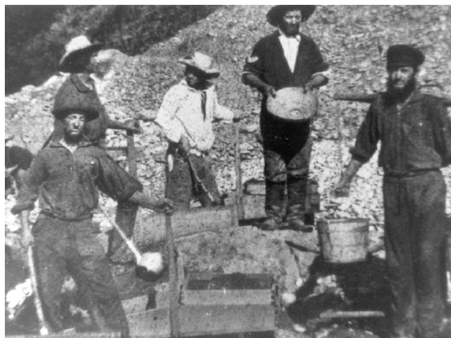
Photo 2. Rockers and gold pan used in California, 1849. Photo courtesy of the Bancroft Library.
