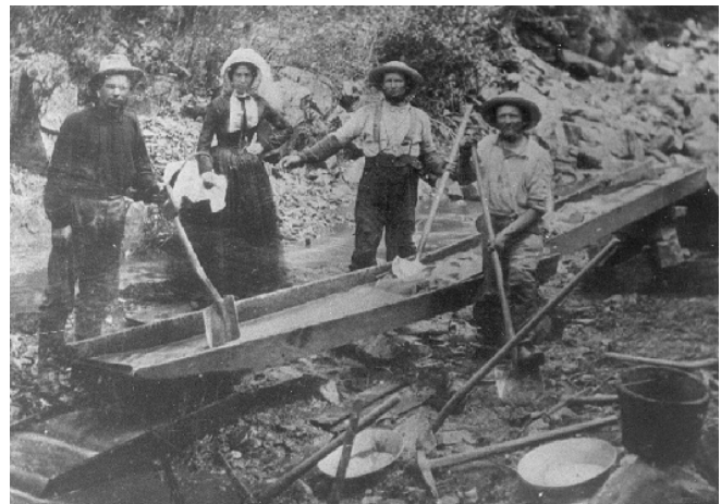
Photo 5. A long tom in use near Auburn, California, early. Photo courtesy of Wells Fargo Bank History Room.
