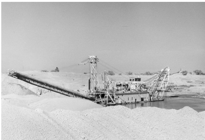
Photo 12. A view of the dredge operated by Yuba-Placer Gold Company. The hull is 223 feet long and the total length is 453 feet.
