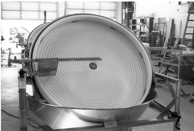
Photo 7. A PMX rotary concentration table. Note the wash water bar with individual jet controls and the concentrate discharge hole in the center.
