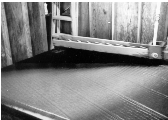
Photo 16. Deister shaking table inside the structure of Photo 15. Note dark bands of separated concentrate to the left.
