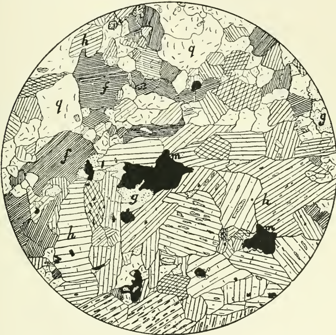
FIG. 69. THIN SECTION SHOWING FREE GOLD IN DIORITE FROM MASHONALAND ( Spurr ). × 25; f . feldspar; q . quartz; e . epidote; h . hornblende; m . magnetite; g . gold.
