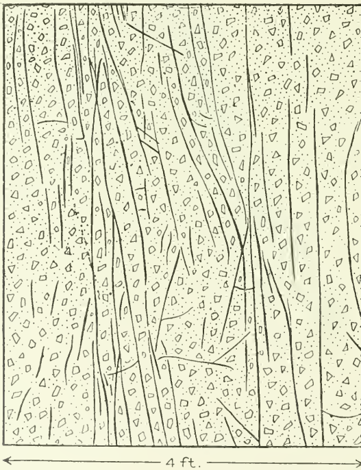
FIG. 185. SHEETING IN BRECCIA, CAPTAIN VEIN, PORTLAND MINE, CRIPPLE CREEK ( Lindgren ).
