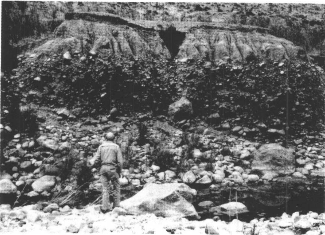
FIGURE 2. — Typical placer material showing the wide variation in particle sizes to be dealt with in sampling.
