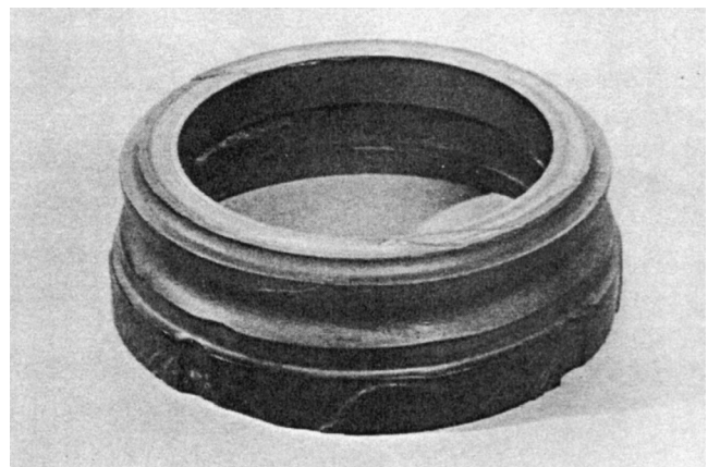
Figure 14. Damage to Outside Diameter of a Seal from Erosion.
