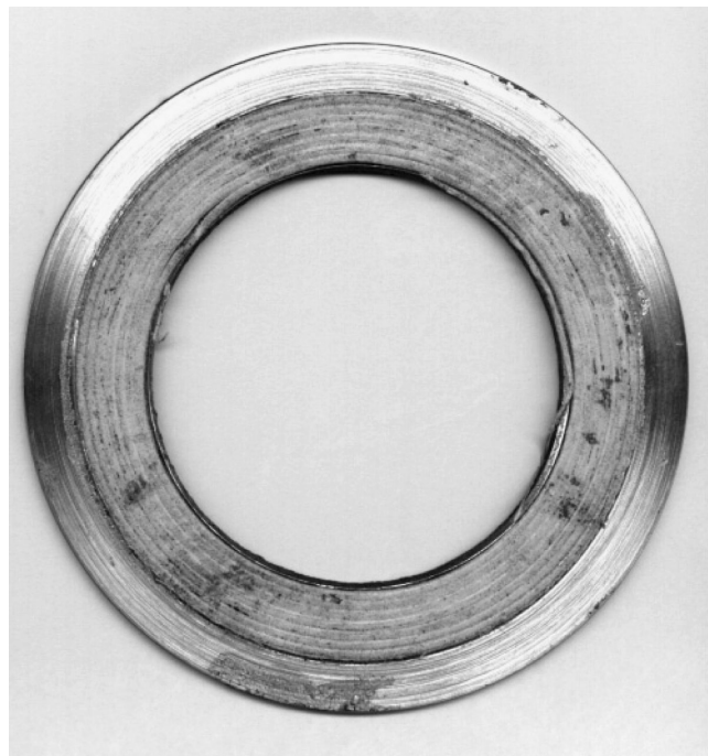
Figure 11. Serrated Metallic Core Faced with PTFE after Compression to 500 MPa.
