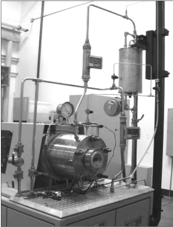
Figure 16. Seal test unit used for EC testing
