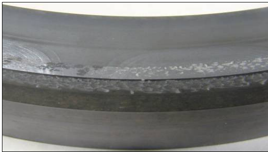
Figure 35. EC damage on fine grain self-sintered SiC rotating face, operated without a ground wire
