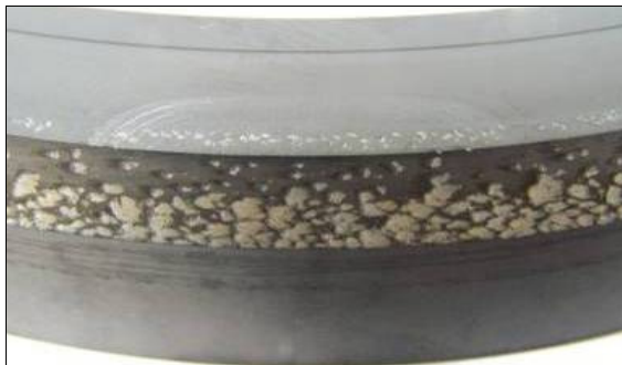
Figure 36. EC damage on \alpha -SiC bi-modal rotating face, operated with a ground wire
