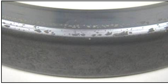
Figure 27. Fine grain SiC rotating face tested at 55 °C
