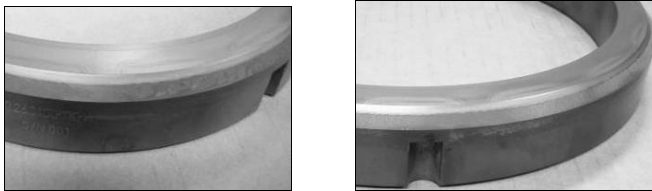
Figure 32. EC damage using full electrically conductive set up
