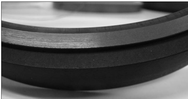
Figure 38. Grainy texture rotating carbon graphite seal face
