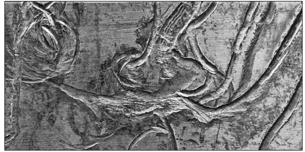
Figure 4. Metal part damage from electrical activity
