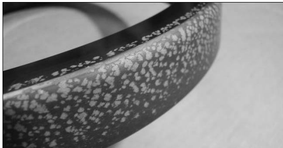
Figure 29. \alpha -SiC bi-modal SiC rotating face tested at 55 °C
