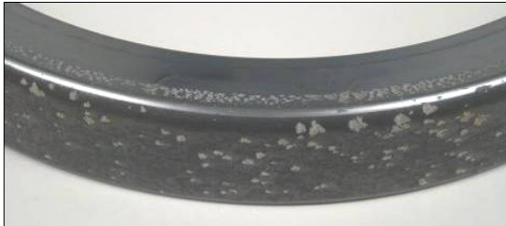
Figure 28. \alpha -SiC bi-modal SiC rotating face tested at 30 °C
