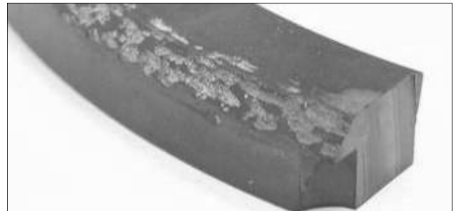
Figure 18. Rotating SiC seal face after 12 months in BWR operation
