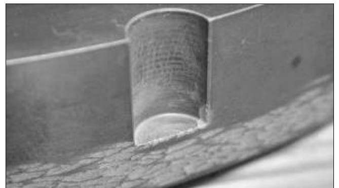
Figure 19. Same SiC seal face material tested 184 hours under benchmark laboratory conditions
