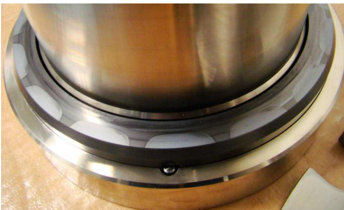
Figure 19. Post-Test 6" Seal Design Wavy SiC Face
