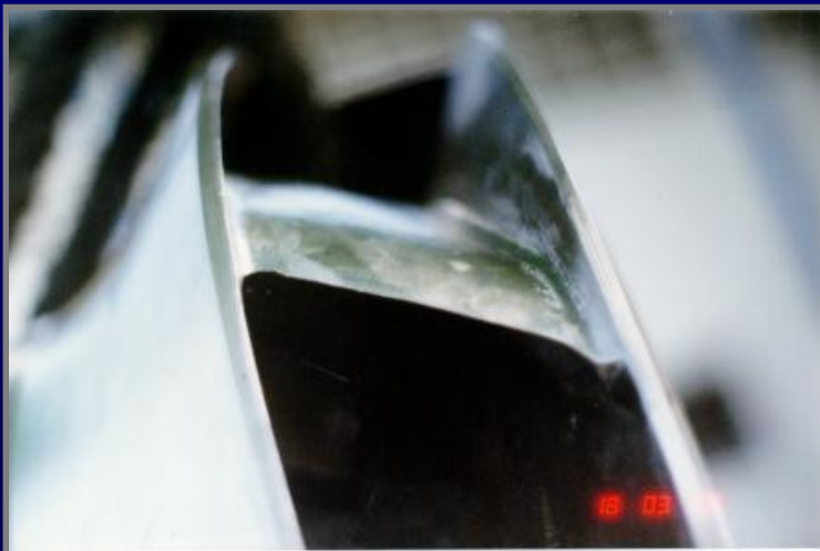
ADJUSTED (UNDER/OVERFILLED) VANE EXIT
