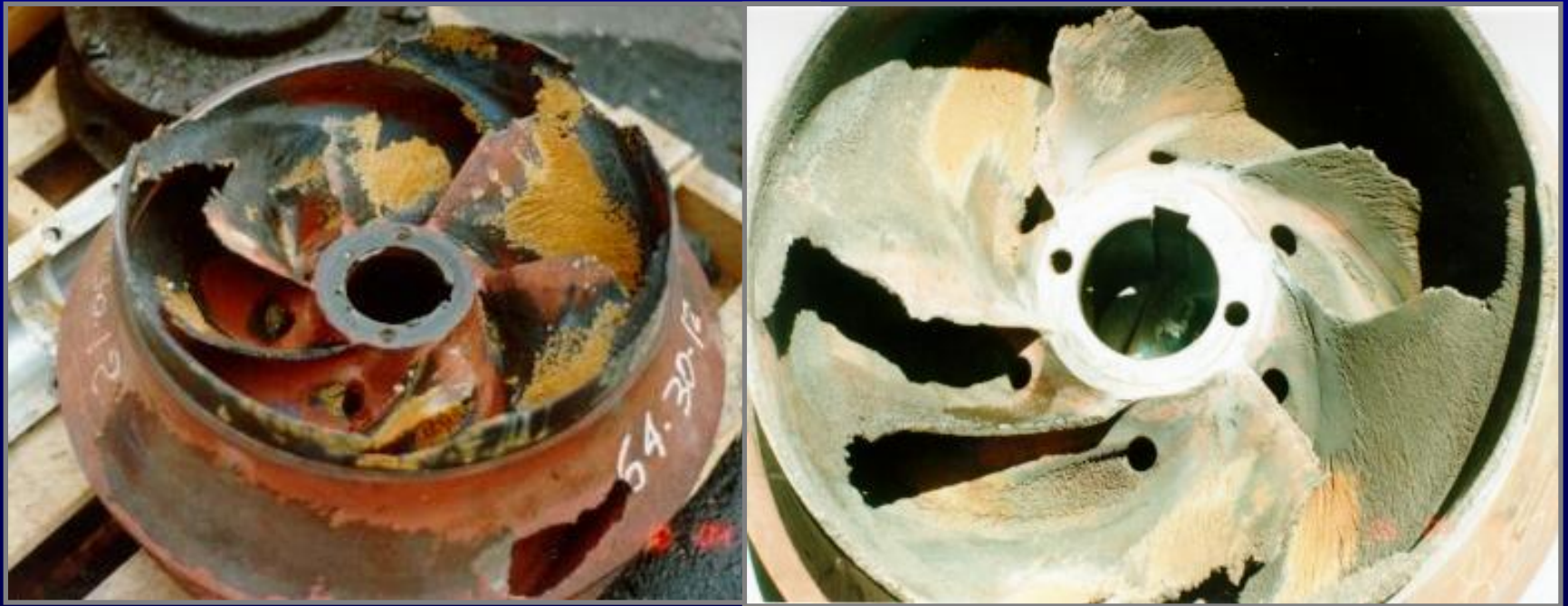
IMPELLER CONDITION AFTER 1 YR IN SERVICE
