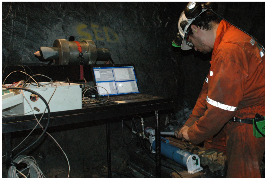
Figure 2 – Testing in the biaxial chamber.
