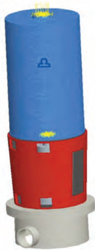
Figure 39. FEA Model for the Canned VTP with \frac{1}{2} Inch (12.7 MM) Thick Plate.
