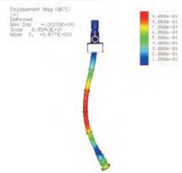
Figure 22. FEA Predicted Second Below-Ground Bending Mode Shape at 3.9 Hz.
