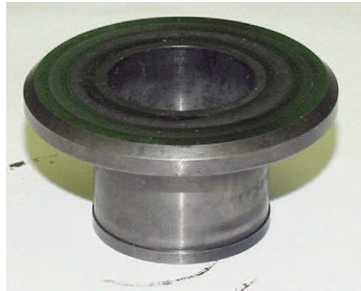
Figure 10. Original “Top Hat” Secondary Seal Rotating Face/Sleeve.
