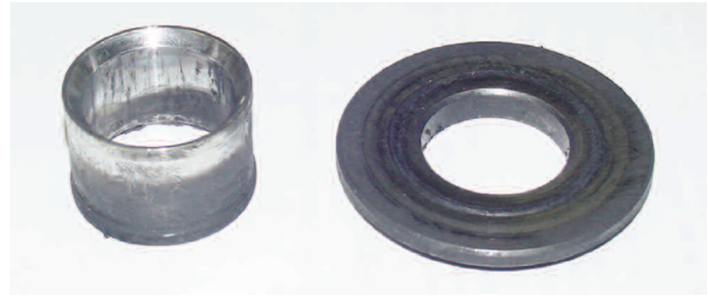
Figure 14. Two Piece Secondary Seal Rotating Face and Sleeve.
