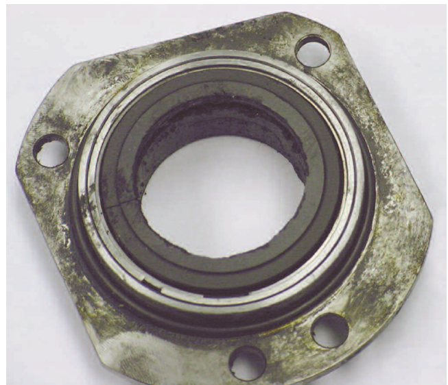
Figure 5. Secondary Seal Stationary Face, Evidence of Dry Running/Cracked Face.
