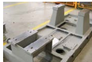
Figure 5: Sloped deck plate mounted between the side rails and extending only under pump and coupling
