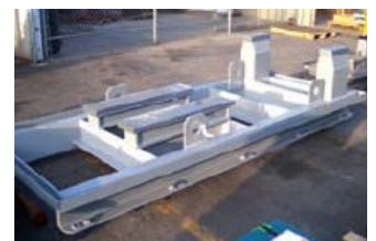
Figure 6: Open deck of the three basic designs with no deck/top plate (grouted or non-grouted)
