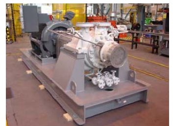
Figure 4: Sloped deck plate between the side rails and extending beneath the pump and driver
