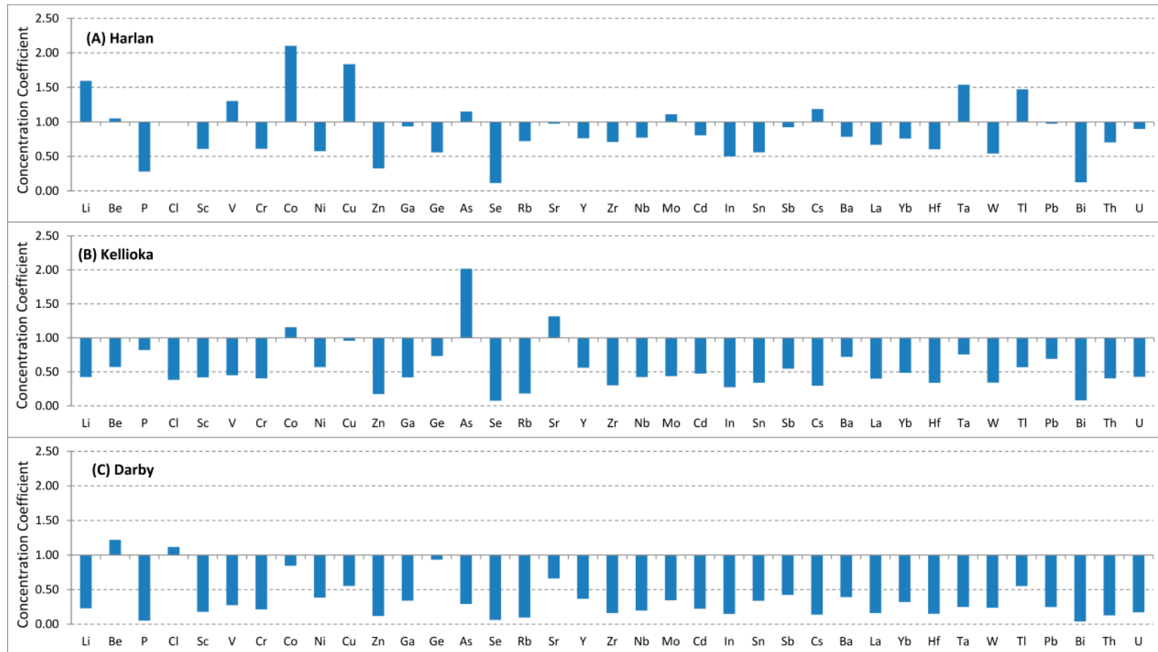
Figure 4. Concentration coefficients of trace elements in the coals studied. (A) Harlan; (B) Kellioka; (C) Darby. Concentration coefficients (CC) are the ratio of the trace-element concentrations in the coal samples vs. world hard coals reported by Ketris and Yudovich [26].
