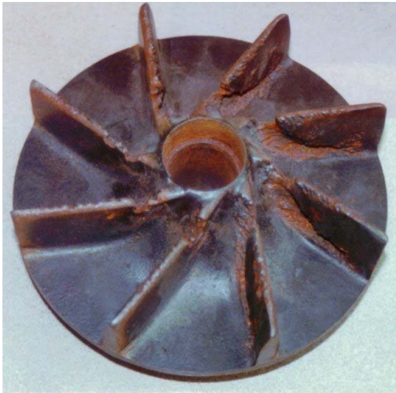
Figure 8 Impeller damaged by cavitation.
