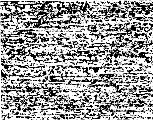
Figure 16. Banded Structure in Medium Carbon Steel Shaft, Attributable to Inadequate Hot Work.
