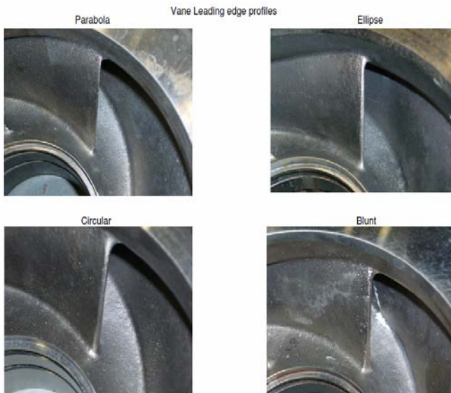
Figure 5: Cast Impellers with different leading edge profiles
