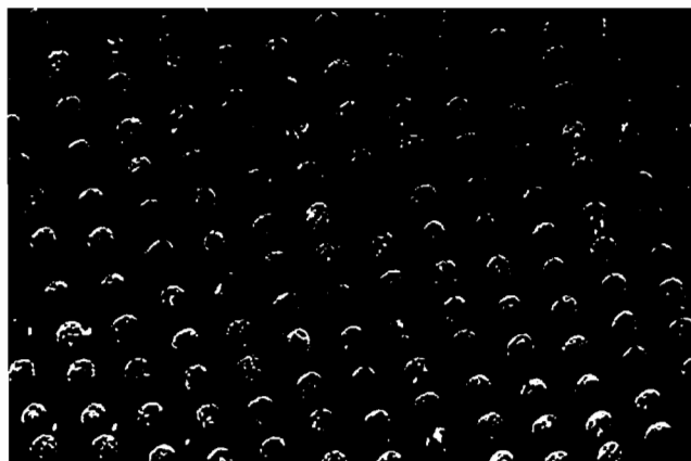
Figure 1. Regular Microsurface Structure in the Form of Micropores.
