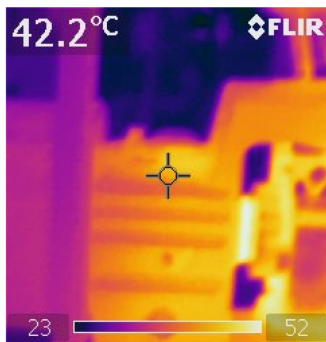
Figure 20. Combined Bearing at 3380 rpm, 621 gpm (141 m³/h).
