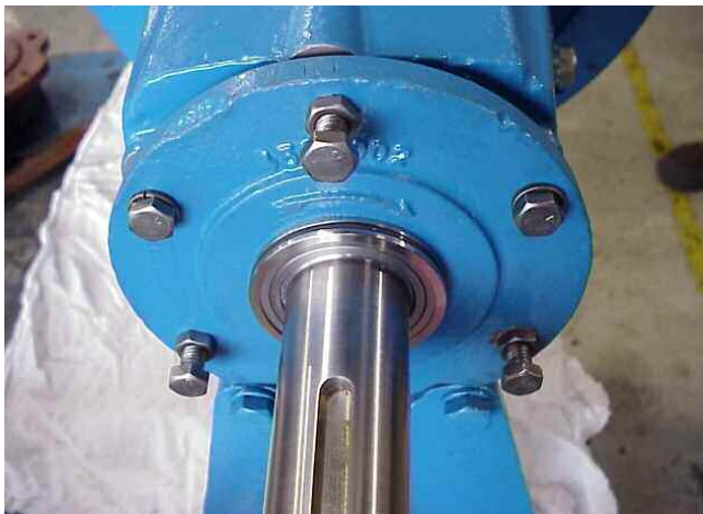
Figure 20. Dual-Face Magnetic Isolator Installed on Bearing Frame of Sump Pump. (Courtesy DanHart Inc.)
