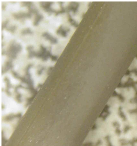
Figure 15. New Dynamic O-Ring from Compound Labyrinth Isolator.
