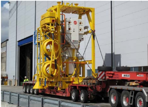
Figure 9. View of a complete Hybrid Pump Module (Courtesy of Pazflor Project)
