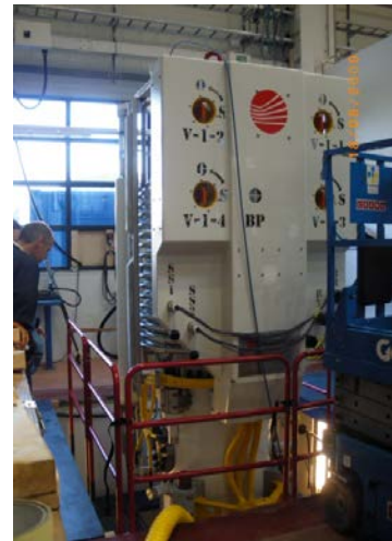
Figure 7. Pump Module Integrity Test (Courtesy of Pazflor Project)
