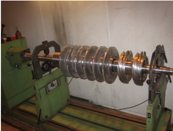
Figure 1. View of the Hybrid pump rotor (Courtesy of Pazflor Project)
