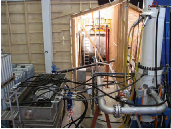
Figure 18. View of the First Pazflor Hybrid Pump on the Test Stand.
