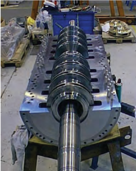
Figure 2. Manufacturer 2 Liquid Booster. (Courtesy of Aker)
