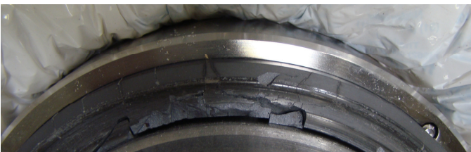
Figure 2: Rotating Face Damage
