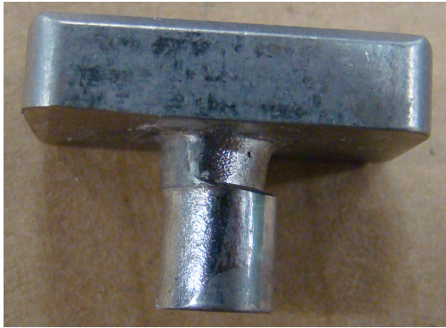
Figure 5: Pin Damage from High Frequency Vibration
