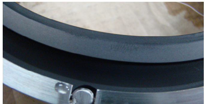
Figure 16: Post-Test Thrust Balance Seal Stationary Face
