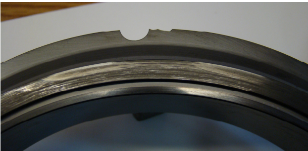
Figure 17: Test Seal Stationary Face After Slow Roll Testing
