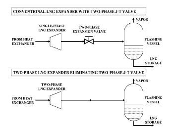
Figure 11: Conventional Single-Phase Versus Two-Phase LNG Expander
