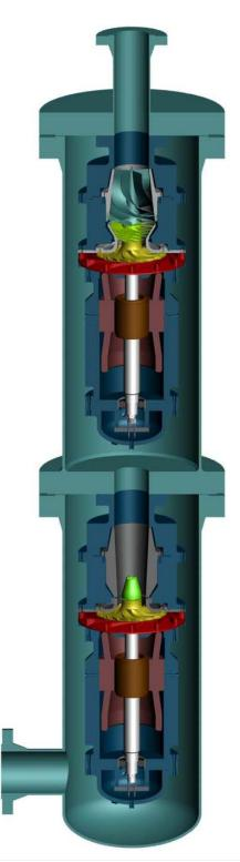
Figure 20: Combined Single and Two-Phase LNG Expanders in Tandem Configuration
