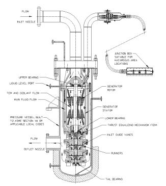
Figure 9: Complete Assembly of an LNG Expander with Downward Flow Design
