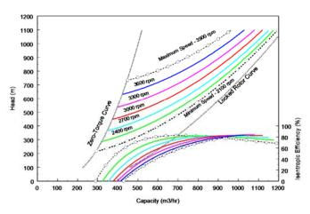
Figure 6: Variable Speed Expander Characteristic
