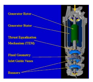
Figure 5: Cross Sectional Drawing of the Variable Speed LNG Expander
