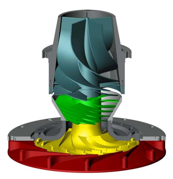
Figure 16: Hydraulic Assembly for Two-Phase Expansion
