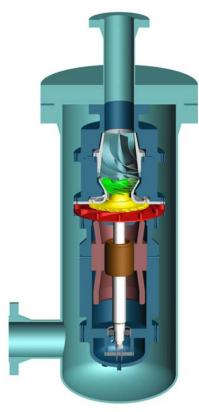
Figure 15: Cross Section of the Two-Phase LNG Expander
