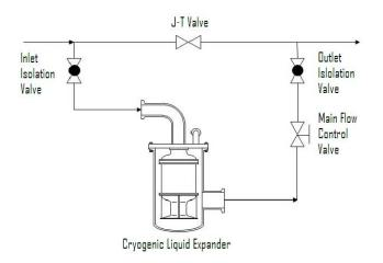
Figure 8: Typical Installation Schematic for an LNG Expander
