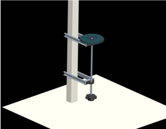
Figure 19: Solid model of the lab static test assembly, with a rigidly mounted flywheel reaction mass. The flywheel was replaced with a flexibly coupled (relatively rigid coupling) motor rotor for the strain gage telemetry tests. This CAD model shows Impeller 1 mounted to the shaft.
