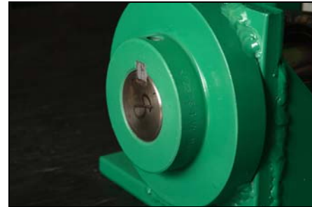
Figure 5c. Fixed end showing interference key installed to prevent rotation slippage under torque load.
