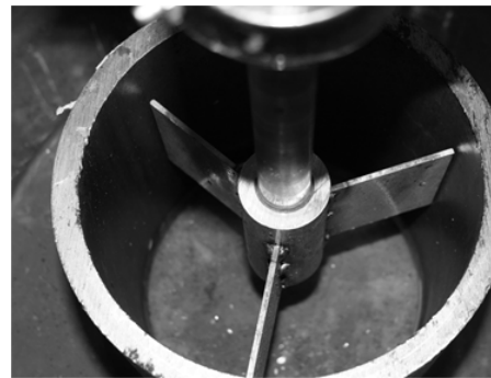
Figure 24: Lab test assembly showing Impeller 5 with straight “paddle wheel” vanes, shown inserted within the stationary shroud.
