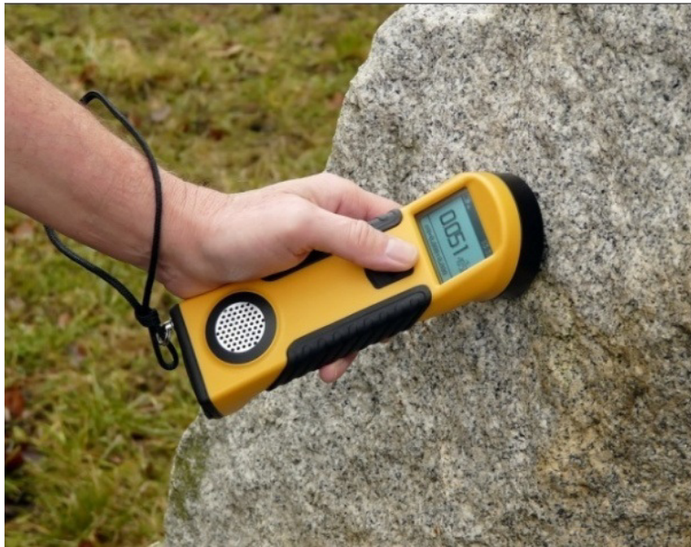
Figure 2 – The hand-held magnetic susceptibility meter (Georadis s.r.o. & Terraplus Inc.)
