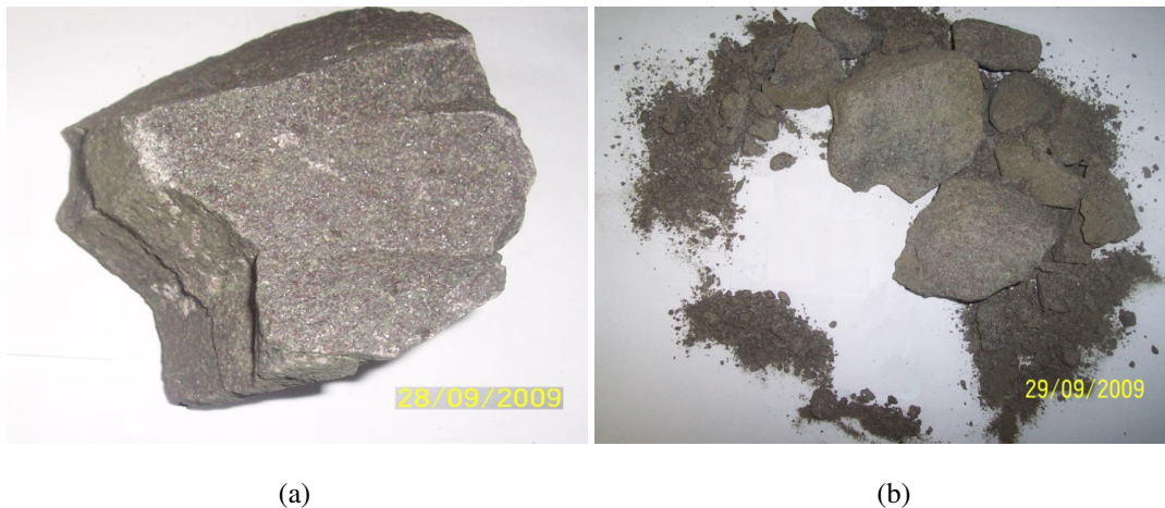
Figure 4 – Results of the glycol test. (a) before the glycol test, (b) after the glycol test (Glycol test=69.73%, LOI=2.57 wt%, Magnetic susceptibility= 1.55 \times 10^{-3} SI Unit)
