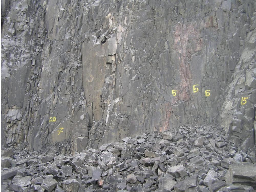
Figure 5 – Field test. Numbers are referring to magnetic susceptibilities of the bench's wall. Magnetic measurements were taken nearly every 10 cm along each bench's wall
