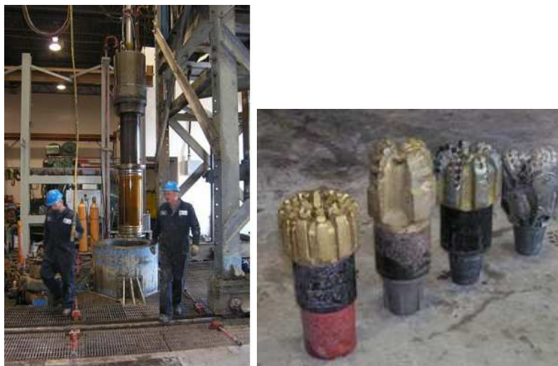
Figure 1 – View of drilled sample lifted out of a pressure vessel (left) and the bits used for drilling (Black & Judzis, 2006).
