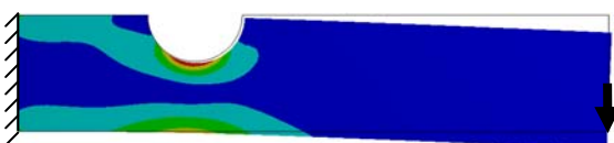
Figure 4: Onset of Yielding with an Applied End Force
