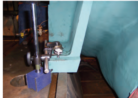
Figure 11. Pump Feet with Dial Indicator.
