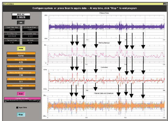
Figure 12. Screen Dump of Enveloped Hydrophone Signal Acquired During Cavitation. (The synthesized envelope is shown over the original filtered signal on the bottom trace. The simple enveloping algorithm converts cavitation bursts into a signal suitable for statistical evaluation and potential for damage.)
