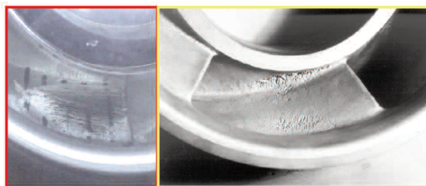
Figure 1. Cavitation and its Effects on a Centrifugal Pump Impeller. (A consequence of cavitation in high-energy pumps, shown in the left view, is the erosion pattern seen in the right hand view.)
