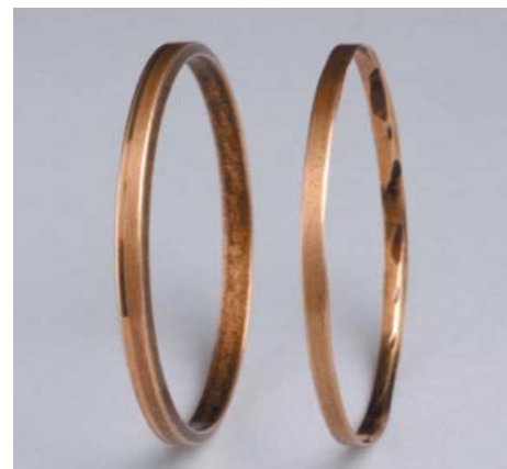
Figure 7. Oil rings in as-new (wide and chamfered) condition on left, and abraded (worn narrow and now without chamfer) condition on right side (Bloch, 2011; Bloch, 2010; Bloch, 2009).
