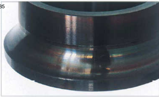
Figure 8. Discoloration from Heat Generation Due to Too Little Lubrication 2
