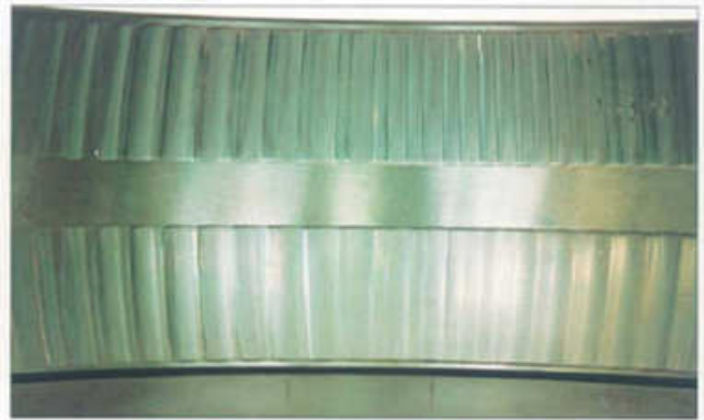
Figure 6. Wear Due to Vibration of a Stationary Shaft 2
