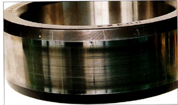
Figure 17: Axial Indentations and Scratches on the Raceway from Roller Contact During Mounting 2
