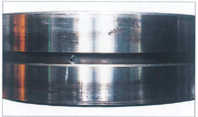
Figure 14. Fretting Due to Loose Fit between Outer Ring and Housing 2
