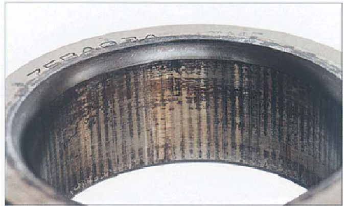
Figure 15. Fretting Due to Insufficient Interference Fit 2
