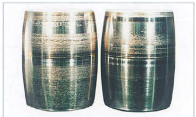
Figure 7. Smearing from Poor Lubrication 2
