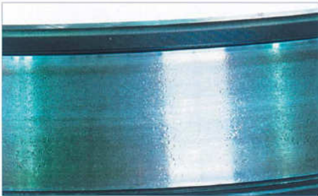
Figure 3. Soft Debris Denting on Raceway 2
