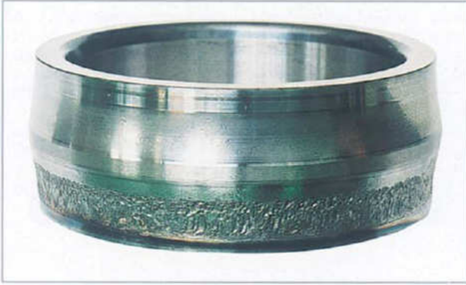
Figure 12. Flaking Due to Excessive Axial Load 2
