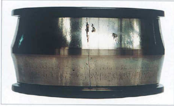
Figure 16. Crack from Large Fitting Stress Due to Temperature Difference between Shaft and Inner Ring 2
