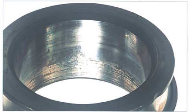
Figure 13. Fretting Due to Insufficient Interference Fit 2
