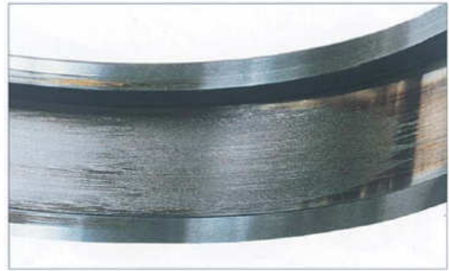
Figure 9. Smearing from Roller Slippage Due to Excessive Grease Filling 2
