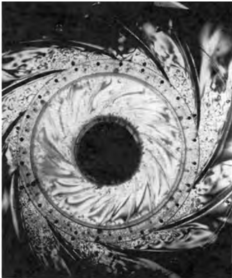
Figure 5. Stalled Flow Visualized Within Pump Impeller and Diffuser at Flow Rates Well Below the BEP. Flow rate is near the rotating stall condition. Whole passages in the diffuser are stalled; others are flowing full. (Courtesy of “Pump Hydraulics—Advanced,” 1999)
