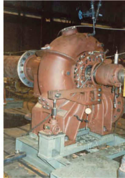
Figure 9. Shop View of the HPRT. The mechanism that actuates the wicket gates can be seen. Otherwise this machine is very much like a pump. (Courtesy of Flowserve Corporation, Pump Division, Taneytown Operation)
