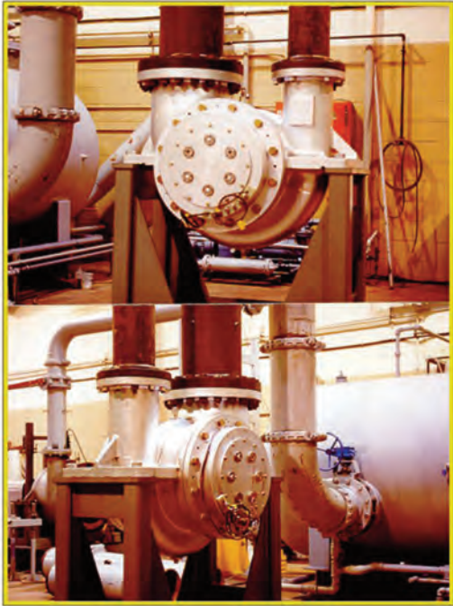
Figure 12. 400 HP, Double-Suction Sealless Integral Motor Pump. This unit has an 18-inch double-suction impeller/rotor diameter and a correspondingly double-sided PM brushless motor. The unit delivers 3000 gpm at 350 ft. Speed is variable up to 2450 rpm, which is 40 percent greater than normal for this flow rate. (Courtesy of Sloteman and Piercey, 2000)
