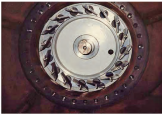
Figure 8. Adjustable Wicket Gates of a Hydraulic Power Recovery Turbine (HPRT). Built by a pump manufacturer as an optimized, variable-geometry turbine instead of a fixed-geometry pump running in reverse as a turbine. (Courtesy of Flowserve Corporation, Pump Division, Taneytown Operation)
