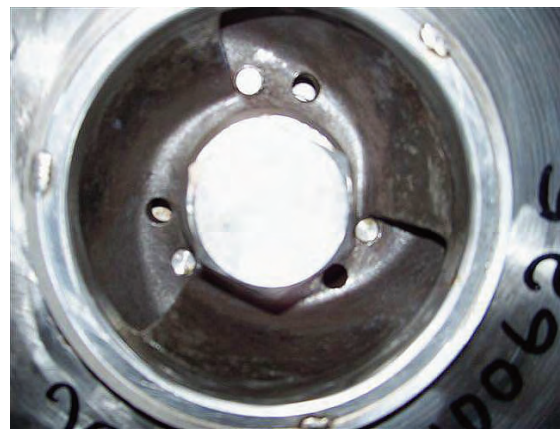
Figure 13. Unfavorable Balancing Hole Design.
