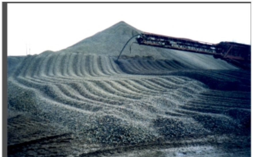
CREATING WINDROWS WITH A TELESCOPING CONVEYOR
