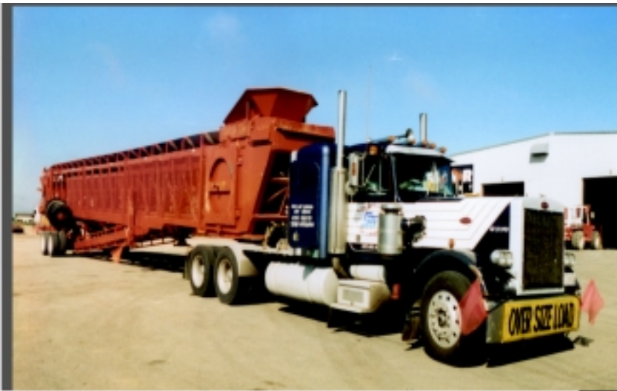
TELESCOPING CONVEYOR READY FOR TRANSPORT
