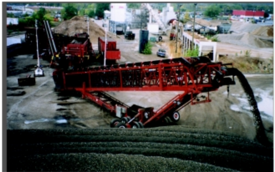
WINDROW STOCKPILING WITH A TELESCOPING CONVEYOR
