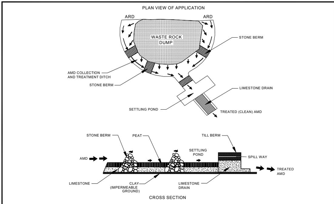
Figure 4. Aerobic- Non Vegetated AMD Treatment System
