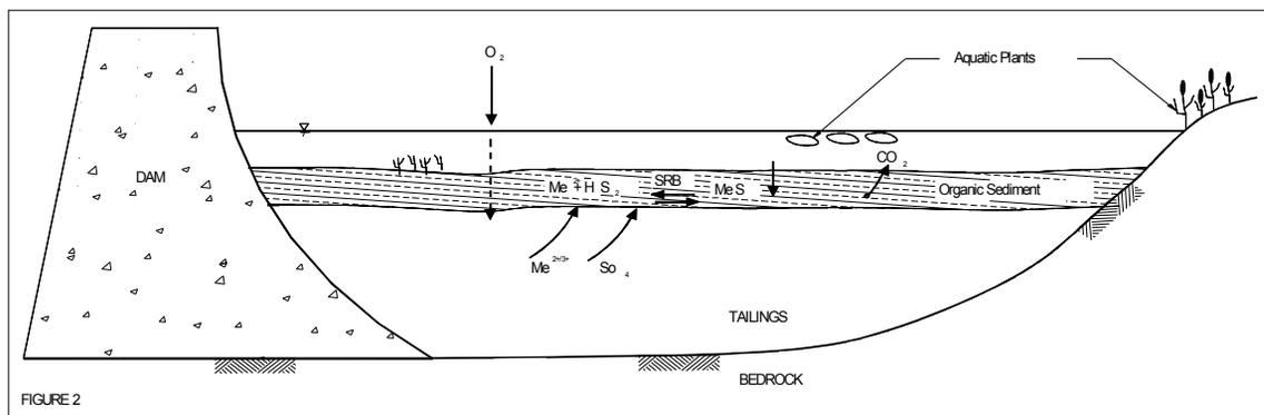
Figure 2. The concept of biologically supported water cover
