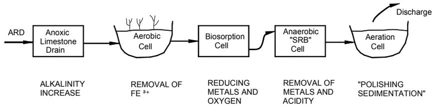
Figure 3. An example of combined passive treatment systems
