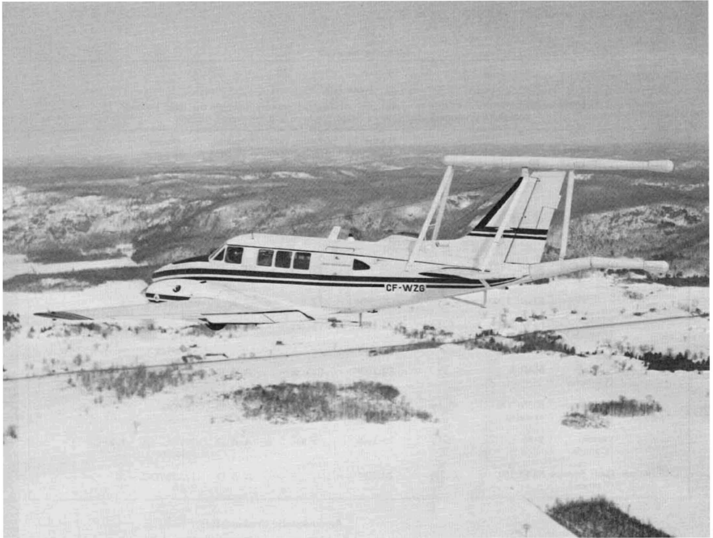
Figure 7.11. Vertical gradiometer system installed on the Beechcraft B80 Queenair aircraft of the Geological Survey of Canada. (GSC 202036-K)
