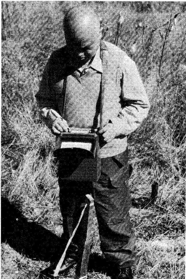
Figure 7.1. McPhar M700 fluxgate magnetometer with strap around operator's neck, being operated on the Cavendish geophysical test range, southwestern Ontario; McPhar Instrument Corp., Willowdale, Ontario. (GSC 202228-G)
