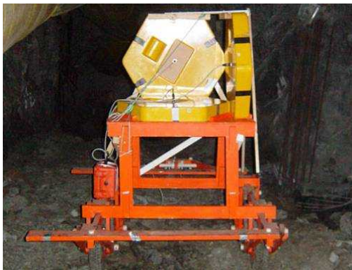
Figure 2: Prototype of the TTEM. Three orthogonal coils (4 plane) are mounted orthogonally on a wooden trailer. Sensitive pre-amplifiers are packed into the boxes on the LHS.
