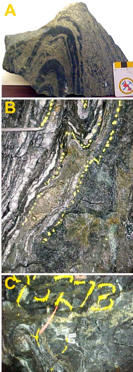
Figure 30: Additional styles of ore in the ID: (A) and (B) are folded massive sulphide bodies and (C) is a conformable and transgressive massive sulphide stringer.
