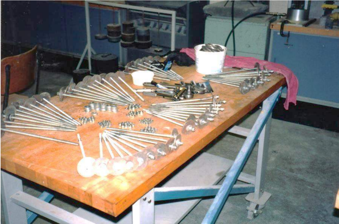
Figure 4: Miniature rockbolts ready for installation.
