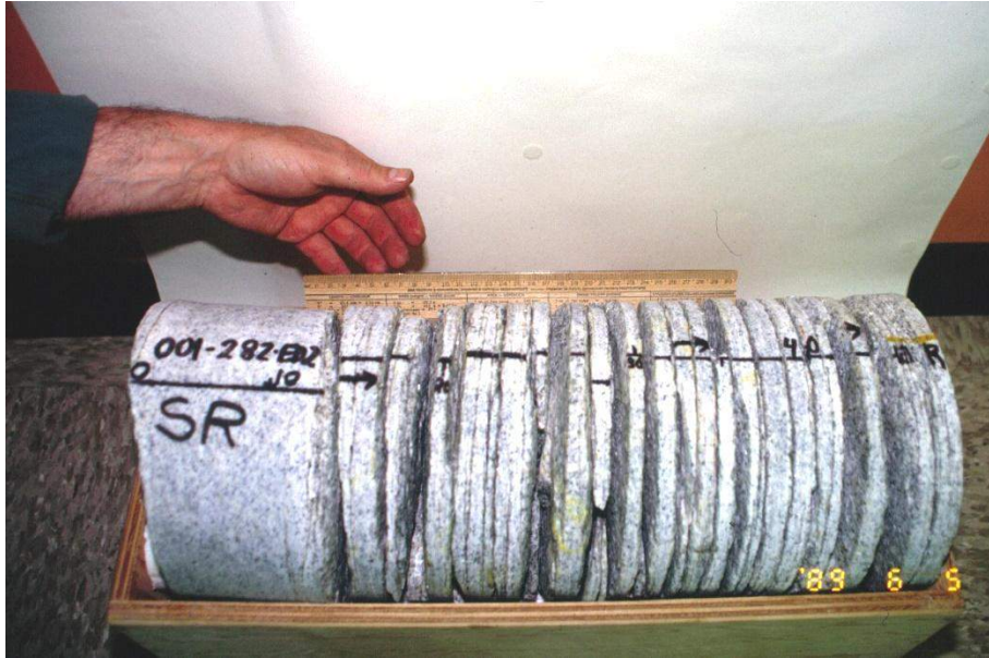
Figure 10: Diking of a 150 mm core of granite as a result of high in situ stresses.
