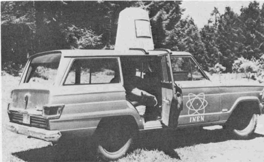
Figure 10C.56. Carborne gamma ray spectrometric survey installation in Mexico (Instituto Nacional de Energia Nuclear) with roof mounted detector. (GSC 203254-I)
