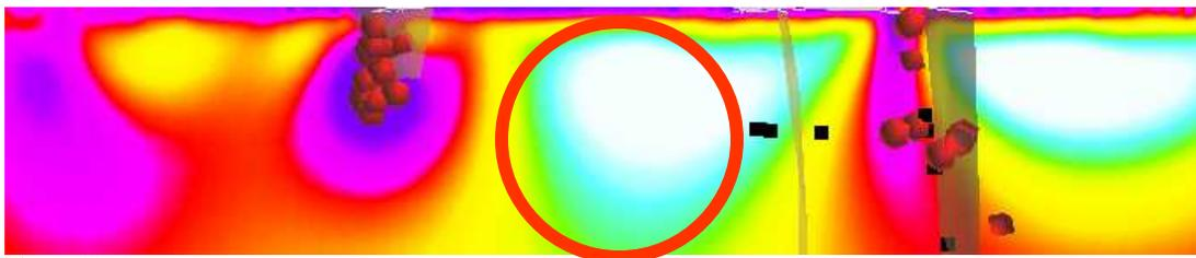
**Figure 11:** Distributed deep earth imaging – resistivity section. 5 km long section, 800 m deep at the Kidd Creek Mine property (a volcanogenic massive sulfide deposit). The survey was able to penetrate thick (50 m) conductive overburden. Data used by permission of Falconbridge and OMET. From Legault et al., 2002.
