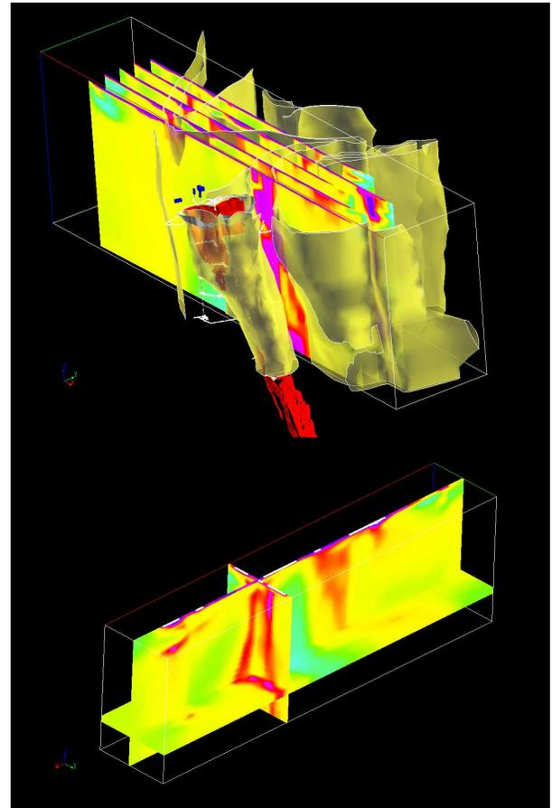
**Figure 9:** (a) Top shows deep MT sections to 2km, (b) bottom shows constrained MT ratioed to the starting resistivity model. Targeting at 1500 metres depth is done utilizing a horizontal slice through the model. at the Kidd Creek Mine and property, near Timmins, Ontario. The study area shown by the cube is 5 km x 1 km by 2 km deep. Data used by permission of Falconbridge and OMET. From Legault et al., 2002.
