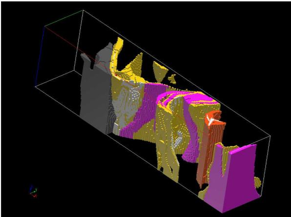
**Figure 8:** (a) Top shows starting geological model, (b) bottom shows physical property model of the resistivity as inferred at the Kidd Creek Mine and property near Timmins, Ontario. The study area shown by the cube is 5 km x 1 km by 2 km deep. Data used by permission of Falconbridge and OMET. From Legault et al., 2002.
