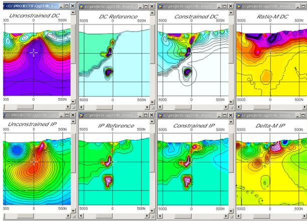
**Figure 7:** Example of constrained inversion results. Deep DCIP data inversions to typical depths of 750 m, DC resistivity on top, chargeability on bottom.
