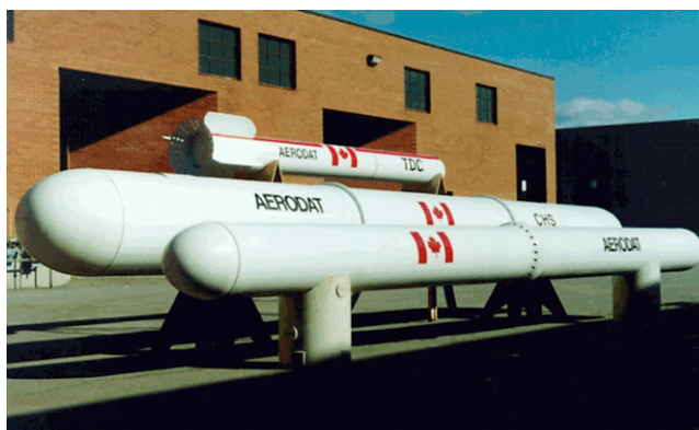
Figure 4: HEM sensor size often depends strongly on the application. Sea ice measurement bird (top), TIBS™ bathymetry bird (middle), and standard 5-frequency bird (bottom).
