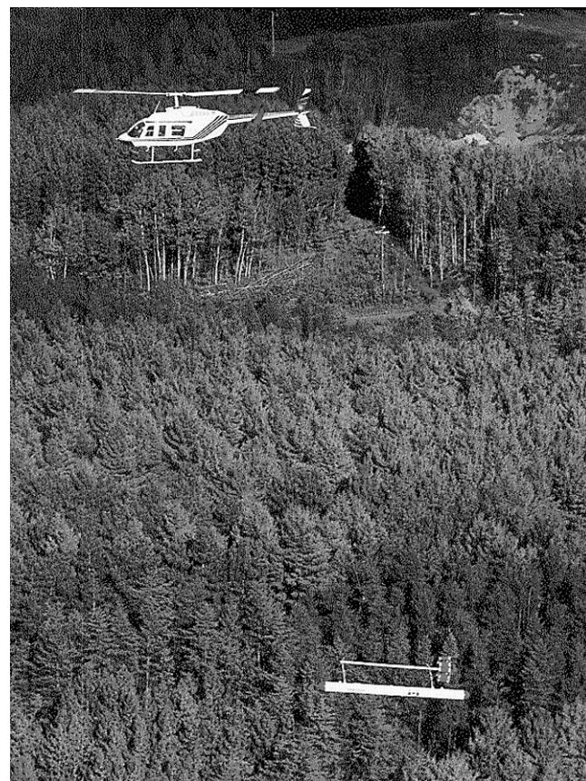
Figure 2: Helicopter Electromagnetic systems. Left: Geonics EM-33, circa 1980, courtesy of Geoterrex; Above: Aerodat 5-frequency HEM, circa 1996. While the general appearance of HEM equipment has changed little since their introduction in the late 1960s, they have become much more sophisticated in terms of their noise, drift and calibration stability over the last ten years.
