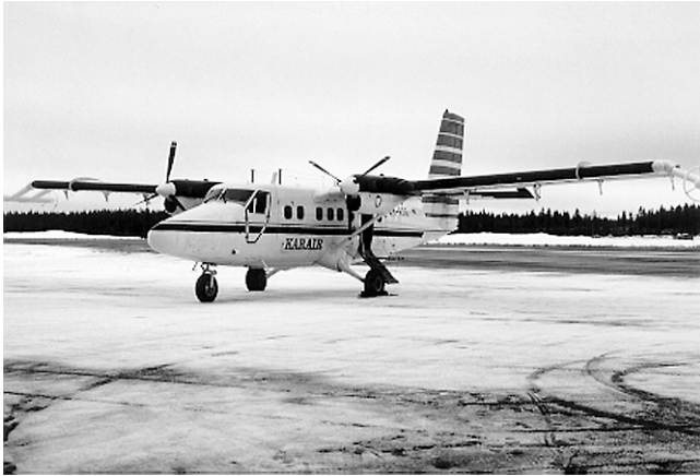
Figure 3: Geophysical Survey of Finland dual-frequency Twin Otter system. Narrowband transmitter and receiver antennas are mounted at the aircraft's wingtips.
