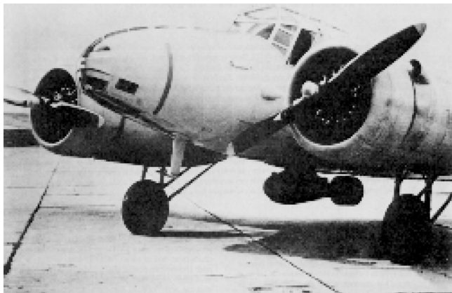
Figure 1: The INCO quadrature system, mounted on an Anson, circa 1954. The transmitter antenna is mounted directly on the wooden skin of the aircraft, while a towed bird (visible below the port engine) housed the receiver coils.
