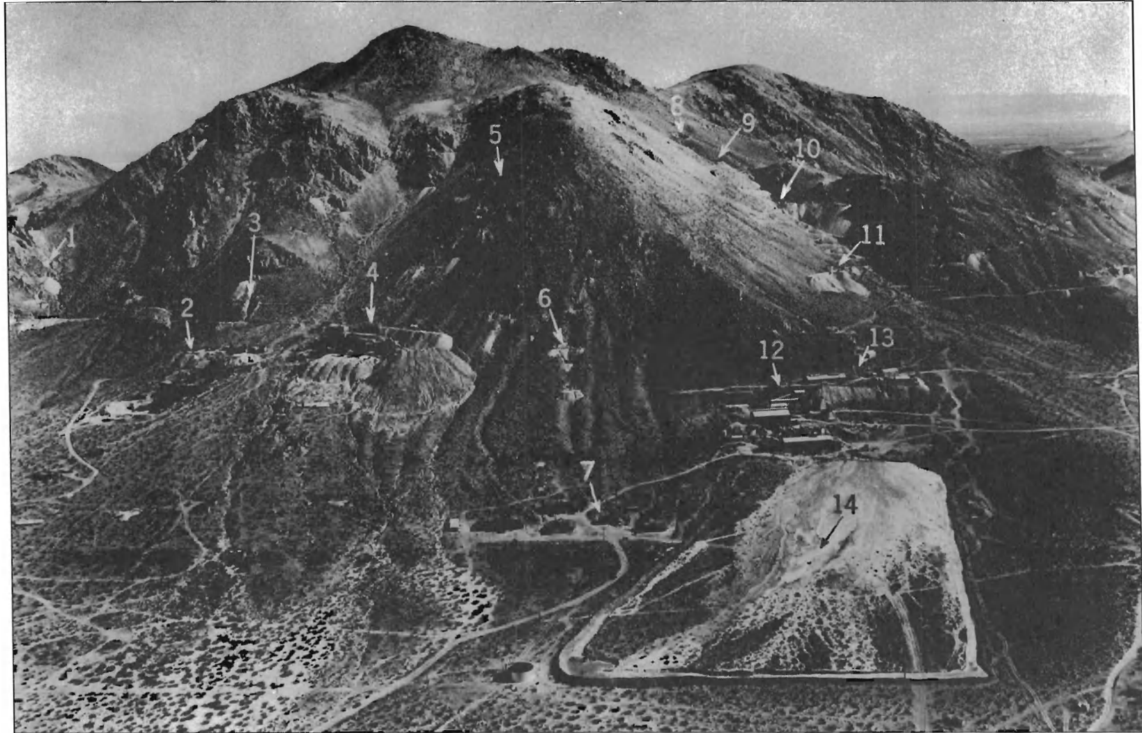
FIGURE 1.- Soledad Mountain from the north: 1, Mojave Mining & Milling Co.'s workings; 2, Karma mill and main haulage adit; 3, Karma open-cut; 4, Queen Esther mill and tailings; 5, Queen Esther mine, caved stopes; 6, Mojave Bonanza workings; 7, Golden Queen office; 8, waste glory hole, Golden Queen; 9, discovery shaft, Silver Queen claim (later Golden Queen mine); 10, adit, 200-foot level, Golden Queen; 11, adit, 400-foot level, Golden Queen; 12, Golden Queen mill; 13, main haulage adit, 600-foot level, Golden Queen; 14, tailings pond, Golden Queen; 15, No. 3 adit, Lodestar.
