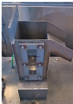
Figure 3.2 JKMRC batch flotation cell used in the laboratory tests.
