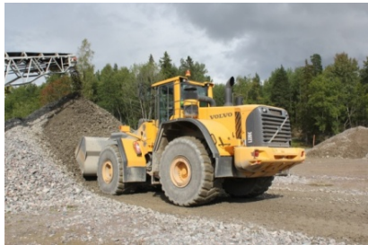
2. Load & Carry (crushed stone)
