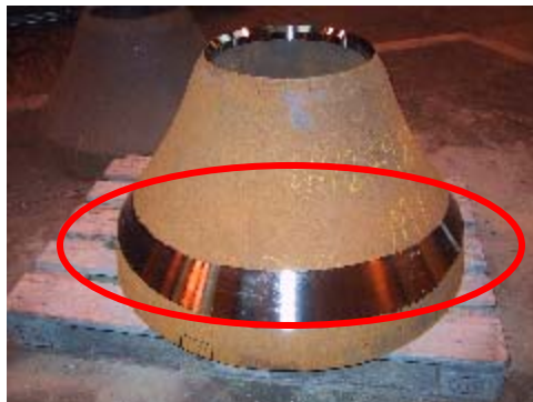
Machining on Original Mantle
