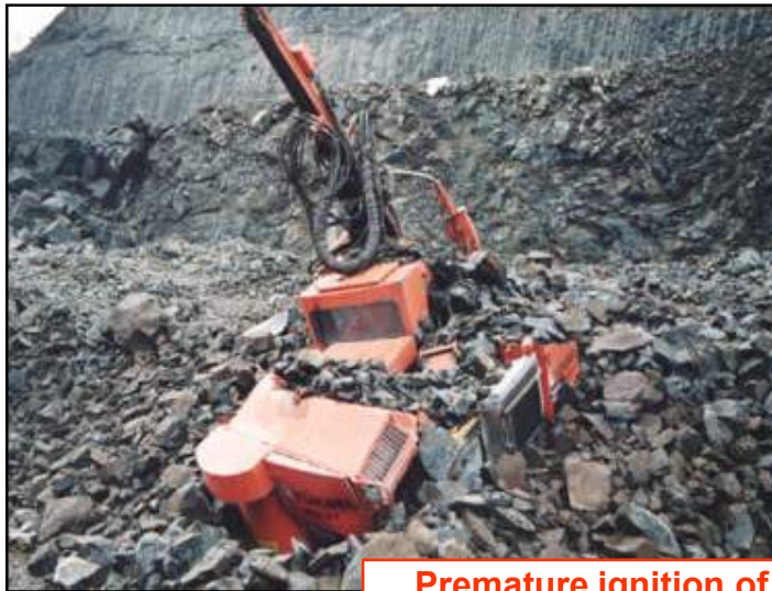
Premature ignition of electric detonators and blast due to lightning
